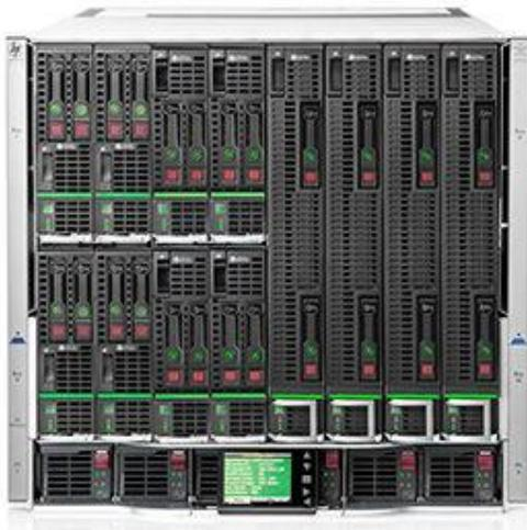
A blade is literally a self-contained server, which collectively fits into an enclosure with other blades. Sometimes known as a chassis, this enclosure provides the power, cooling, connectivity, and management to each blade server. The blade servers themselves contain only the core processing elements, making them hot-swappable. HP refers to the entire package as a BladeSystem.
